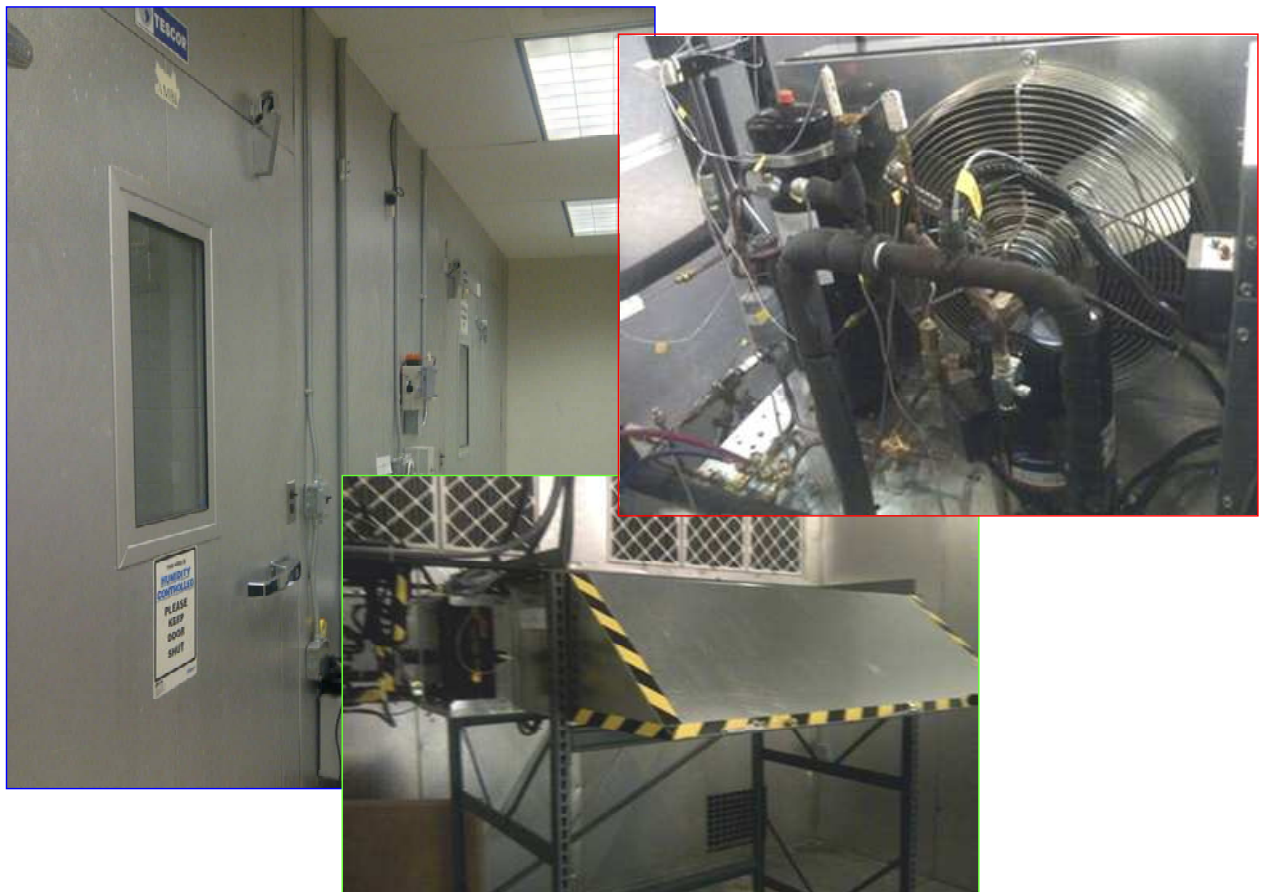
Some pictures of the test equipment: the two chambers on the left, evaporator at the bottom (placed in one of the chambers), and condensing unit on the right (placed in the other one).
