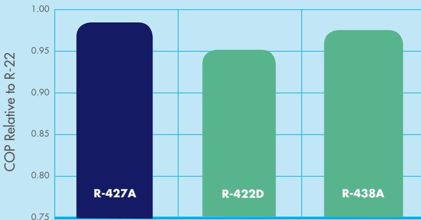
Note: Standard Cycle 100°F Condenser, 50°F Evaporator, 10°F Subcooling and 10°F Superheat
